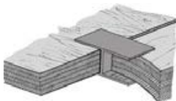
FIGURE 11 - 'H' Clip Detail
