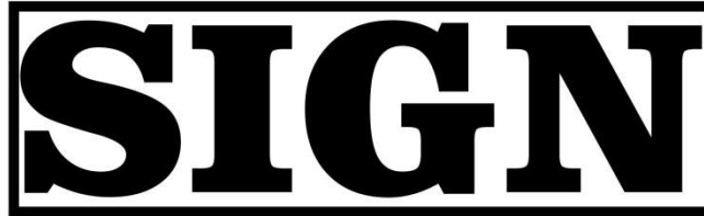
Illustration 1 Sign surface area equals the smallest rectangle surrounding any writing or symbols
