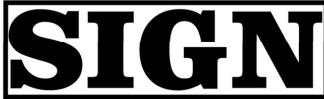
Illustration 7 Sign Surface area equals the smallest rectangle surrounding any writing or symbols
